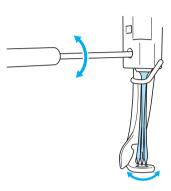
With the flat side of the needle toward the back of the machine, insert the needle all the way up until it touches the needle bar stopper. Pass the needle through the hole in the presser foot, and then use the needle changing tool to lift up the needle.
